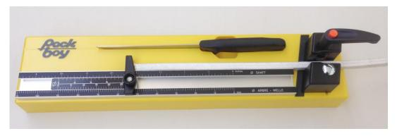
Calibrating and cutting tool for soft packings, for shaft diameter up to 110mm (4 1/4"), with extension scale (optional) up to 250mm (10")
