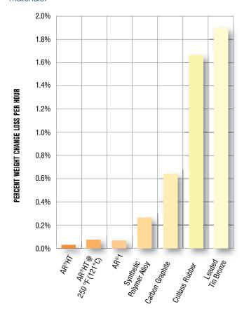
Note: Bearings made from each of the materials (size: 2 in. x 1.5 in. x 1.5 in./ 5.1 cm x 3.8 cm x 3.8 cm) were tested at 900 rpm under 25 psi (0.17 MPa). The run time of the test was eight hours. The test was conducted on 300 series SS shaft, in 95 percent water and five percent silica sand. All materials were tested at  $70^{\circ}$ F ( $20^{\circ}$ C). Additionally, AR®HT was tested at  $250^{\circ}$ F ( $120^{\circ}$ C) in ethylene glycol.
