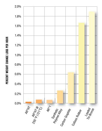
Note: Bearings made from each of the materials (size: 2 in. x 1.5 in. x 1.5 in./5.10 cm x 3.80 cm x 3.80 cm) were tested at 900 rpm under 25 psi (0.172 MPa). The run time of the test was eight hours. The test was conducted on 300 series SS shaft, in 95 percent water and 5 percent silica sand. All materials were tested at  $70^{\circ}\text{F}$  (20°C). Additionally, AR®HT was tested at 250°F (120°C) in ethylene glycol.
