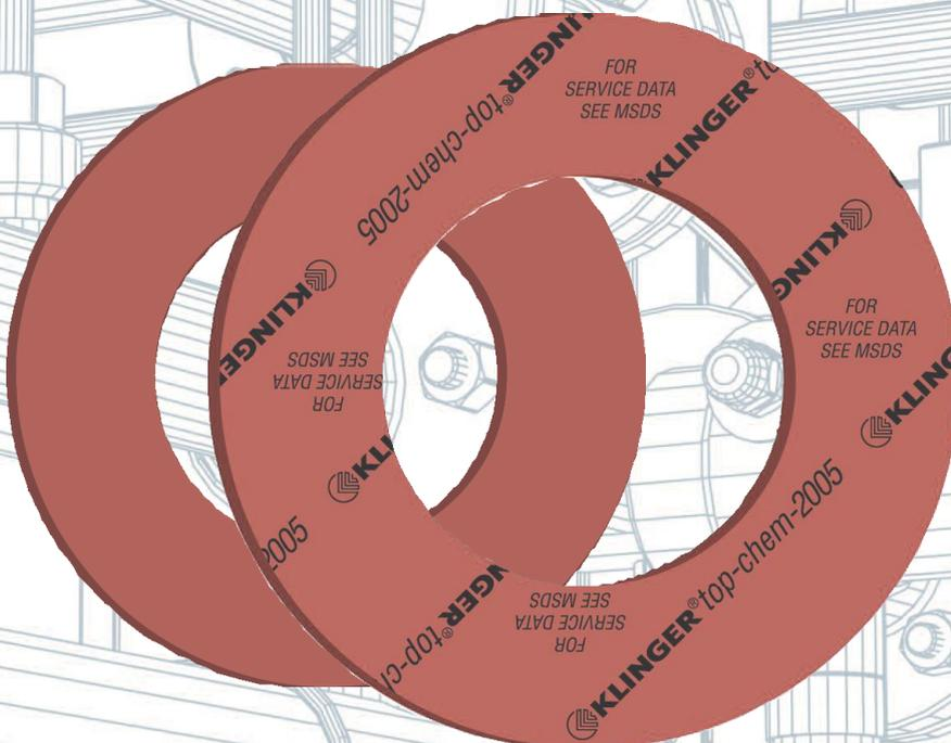
KLINGER®top-chem 2005 PTFE filled with inorganic fillers. Excellent chemical resistance in strongly acidic applications. Suitable for a wide range of applications in the chemical industry. Good mechanical properties at medium temperatures and loads. Economical alternative at the usage of modified PTFE gaskets.
