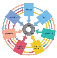
A statement about the expected tightness of the flange connection is only possible if a qualified and defined installation of the gasket has been executed.
