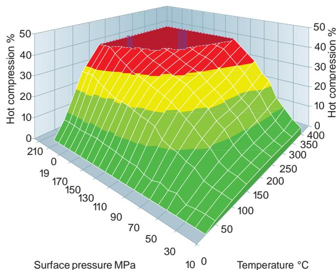
The diagram shows the additional thickness decrease at temperature.
