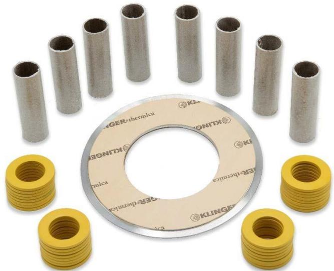
Insulation sets are used to limit corrosion in pipeline systems. Where dissimilar metals are present, the sets remove the possibility of the system acting as a galvanic cell and reduce the risk of galvanic corrosion of the pipework.
