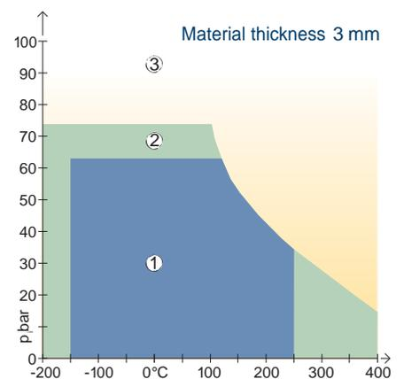
As the maximum operating pressure and load bearing capability are both depending on the gasket thickness, KLINGER provides thickness related pT diagrams.
