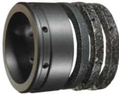
The PackRyt Diverter is a unique stuffing box sealing arrangement that incorporates a flush channel relocation system internally within the composite bearing. This replaces outdated lantern ring/packing configurations that dump excess water into the process. The Diverter relocates the flush deposit and drastically throttles flush volume. Our system ALSO brings shafts into concentricity and keeps them there, significantly increasing sealing reliability.
