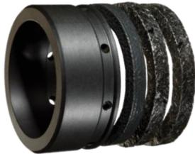
The PackRyt® Sealing System is a unique stuffing box sealing arrangement that incorporates a bearing and flush channel system together. This replaces outdated packing/lantern ring/packing configurations. Our system brings shafts into concentricity and keeps them there, significantly increasing sealing reliability.
