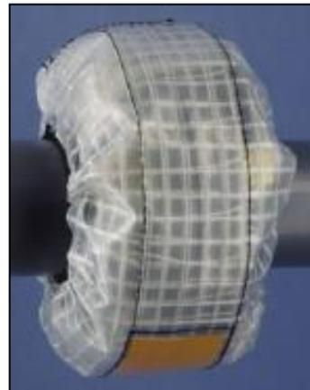
Safety Spray Shields are designed to prevent a catastrophe by temporarily containing hazardous leaks and sprays. Leaks can occur on piping systems conveying chemicals, high temperature fluids, and steam, which can harm workers, damage nearby equipment, and the environment.
