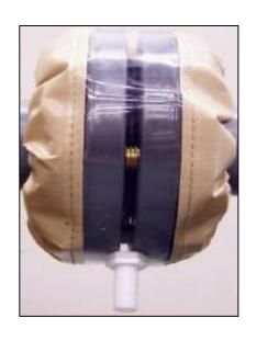
Safety Spray Shields are designed to prevent a catastrophe by temporarily containing hazardous leaks and sprays. Leaks can occur on piping systems conveying chemicals, high temperature fluids, and steam, which can harm workers, damage nearby equipment, and the environment.
