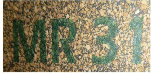
MR 31 Cork is a highly compressible automotive and general purpose gasket material with moderate oil resistance.
